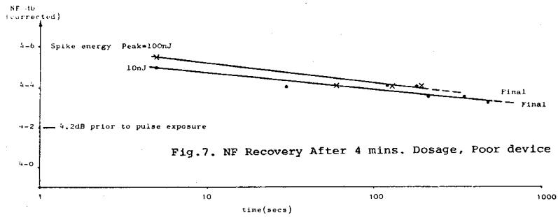
Fig.7. NF Recovery After 4 mins. Dosage, Poor device
