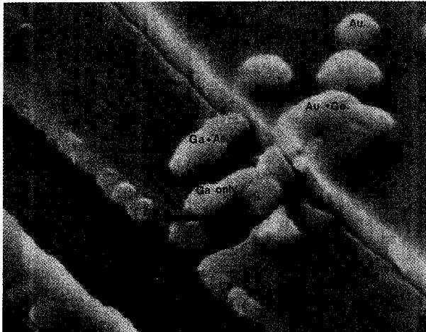
Fig.6. EDAX Examination of Failed Device
