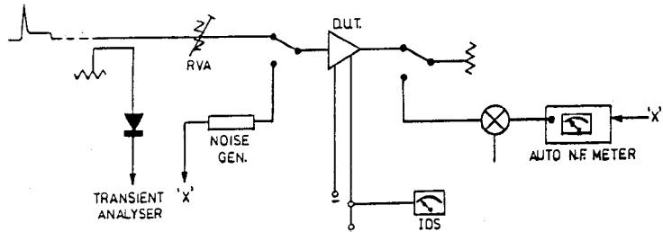
Fig.2. Test Arrangement for Catastrophic Burn-Out
